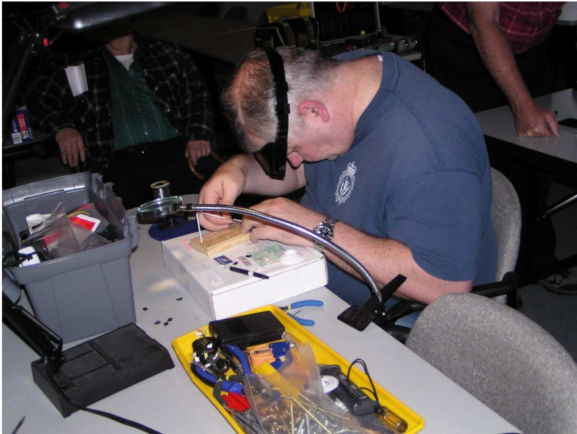
Robert Parker VE3RPF Preparing to solder the microcontroller
